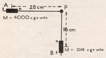
shown. Their magnetic moments are 4,000 and 2,048 c.g.s. units, and the distances from the corner P to their mid-points are 20 cm. and 16 cm. respectively. Calculate the resultant field strength at P.
